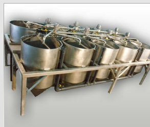
Tank Farms, Corn Soak Systems
