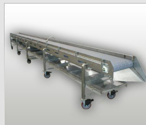
Sanitary Process Conveyor
