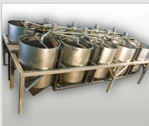
Tank Farms, Corn Soak Systems
