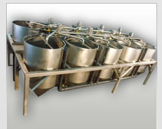
Tank Farms, Corn Soak Systems
