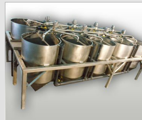
Tank Farms, Corn Soak Systems
