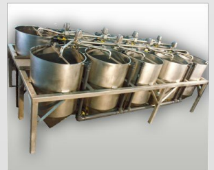
Tank Farms, Corn Soak Systems
