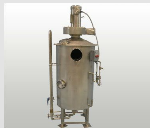
Water Bath Dust Control System
