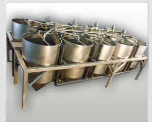
Tank Farms, Corn Soak Systems
