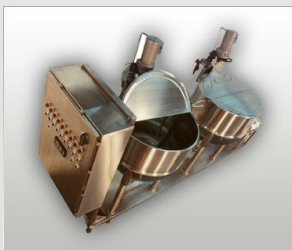
Mixing Use Tank Skid
